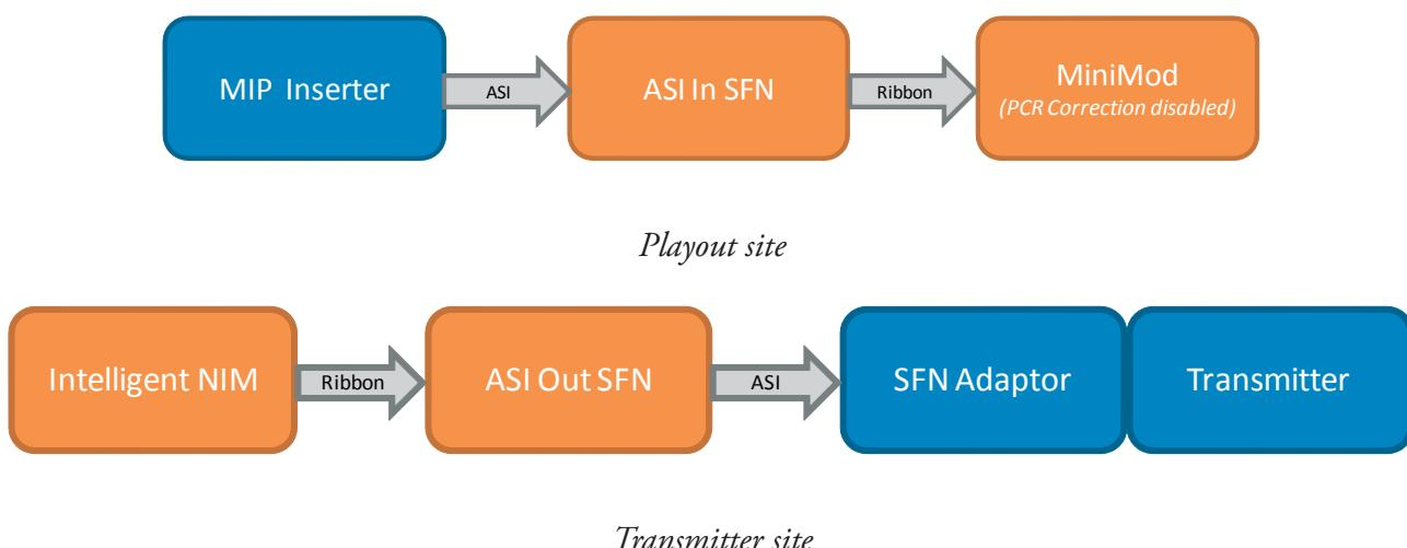
The picture above shows an example setup of using SR-Systems components to transport data from the playout site to the transmitter sites in an SFN network setup.
